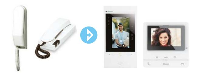
Easy shift from the old analogue audio system to the new 2 Wires colour video system.
