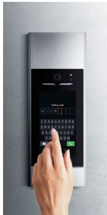
APARTMENT BLOCK/RISER/ FLOOR/ APARTMENT Entering the exact address of the apartment to call in the system.
