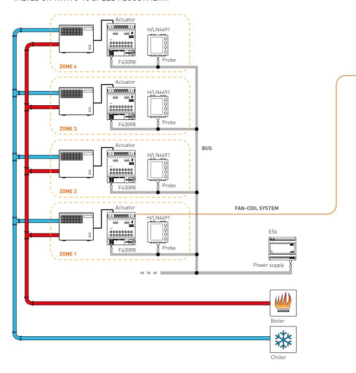
Note: 0-10V valves are not managed in proportional mode, but in ON-OFF mode
