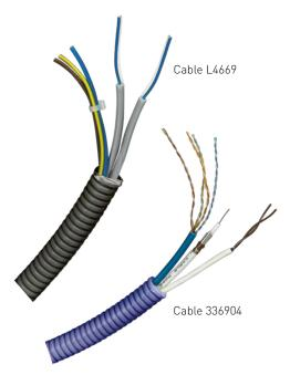
Although the cables guarantee electrical insulation up to 300/500 V, there is no guarantee of immunity from disturbance, which may occur when the cable is installed inside the same conduits as the 230 V power supply cables. These types of installation are strongly NOT recommended in new systems but are permitted in case of refurbishment of the building to save on masonry work.
