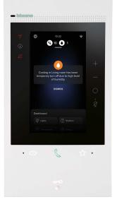
Classe 300EOS with Netatmo: notification of temporary cooling deactivation due to high humidity.
