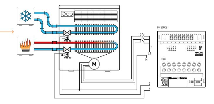
Variation for the connection of a 4-tube fan-coil with 0-10 V speed adjustment - use of two 0-10 V outputs (set LOAD = 3 in case of physical configuration).
