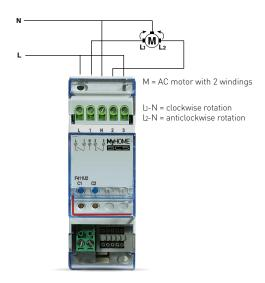
Actuator, item **F41102** with 2 relays for ON/OFF lighting control. In the diagram, the device is wired for the control of a motor-driven shutter, and must be set in "relay interlock" mode.
