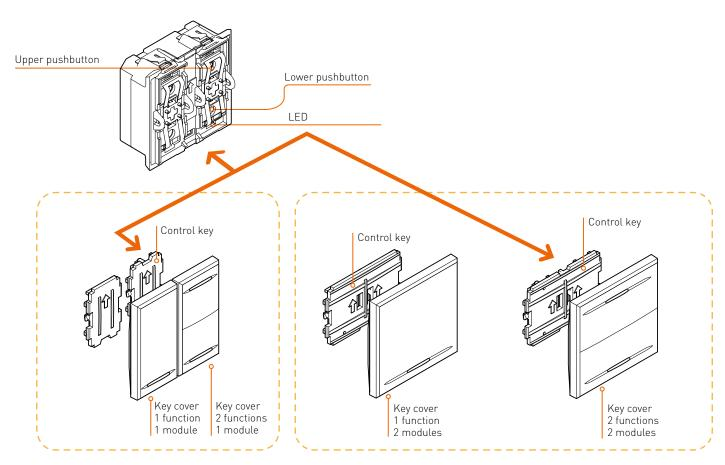
The control with single key cover can be compared with a traditional closing contact (pushbutton or switch).
