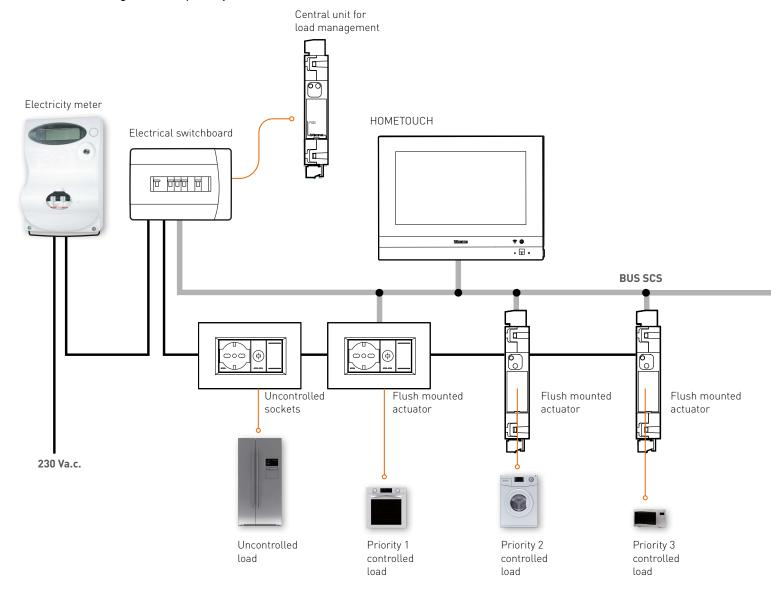
**NOTA:** the load control management central unit is positioned inside the electrical switchboard.
