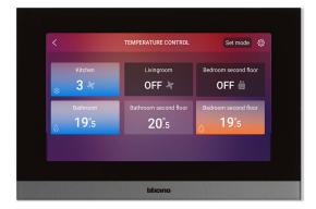
HOMETOUCH: screen with the status of the different temperatures in the rooms and the on/off status of the heating. The orange area shows that the humidity control logic has been activated.
