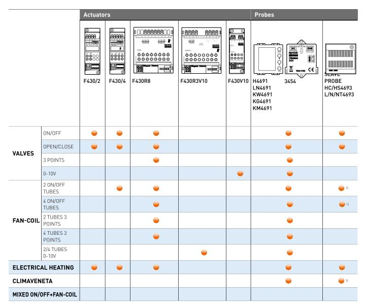
Note 1): Changing the speed using the probes is not possible
