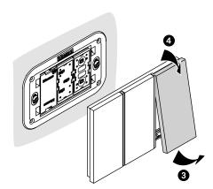
Removal of the control devices from the electrified frame for installation in a different position.
