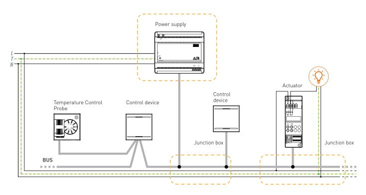
Distributed installation: actuators and control devices are installed in device or junction boxes.
