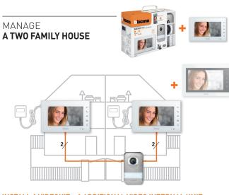
INSTALL 1 VIDEOKIT + 1 ADDITIONAL VIDEO INTERNAL UNIT Add and mix up to 2 additional video internal units
