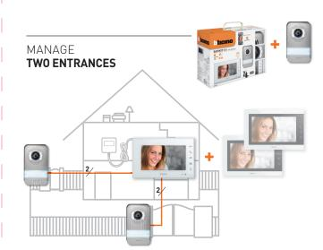
**INSTALL 1 VIDEOKIT + 1 ADDITIONAL ENTRANCE PANEL** Add and mix up to 2 additional video internal units
